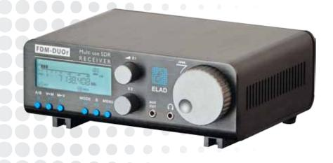
Frequency range: RX 9kHz to 54MHz direct sampling receiver + VHF undersampling reception
